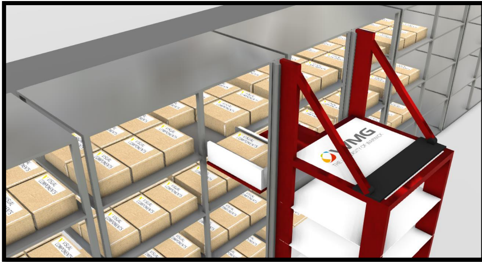
Figure 15 - Self-Stacking Attachment loading Shelves
