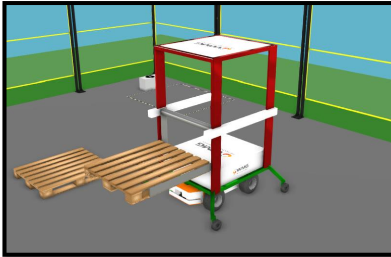
Figure 13 - Pallet Stacking Attachment
